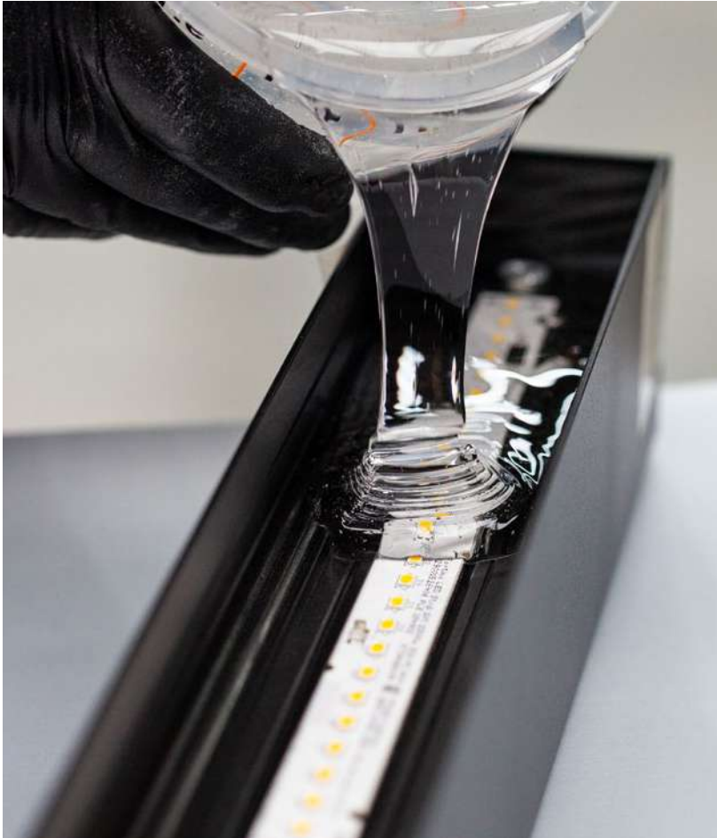
After mounting LED boards into aluminium profiles, a two component, optically clear High Strength Silicone Elastomer is used for IP65 protection.
