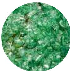
**Recycled glass** is made from waste glass. Glass recycling uses less energy than the production of new glass. Every 1000 kg of waste glass recycled into new items saves 315 kg of carbon dioxide from being released into the atmosphere during the production of new glass. Glass is infinitely recyclable. So keep going to the glass containers on your way to the supermarket!
