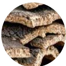
**Cork** is harvested from the trunk of the cork oak *Quercus suber*. The harvesting process does not damage the tree. It is similar to shearing wool off a sheep. Cork oaks are productive for 150 years. Portugal produces 55% of the world production.
